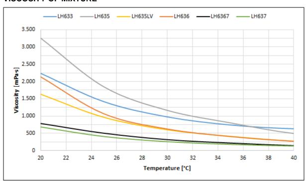
Measuring conditions: Viscometer, cone-plate configuration, diameter 50 mm, gap 0.1 mm
