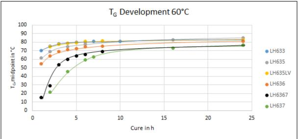
Measuring conditions: DSC-measuring heat rate: 20°C/min, sample mass 10-20 mg
