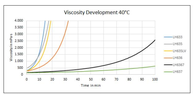
Measuring conditions: Viscometer, cone-plate configuration, diameter 50 mm, gap 0.1 mm
