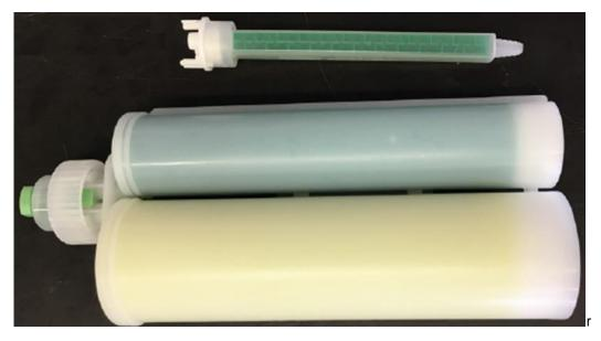
The resin and curing agent components are strongly pigmented in order to make identification of correct mixing possible, especially at the very beginning of the mixing process.
